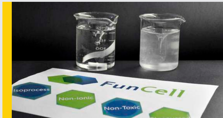
A photo of a paper with (left) and without (right) the additive in stirred water. With the FunCell additive the paper stays intact compare to the other.
