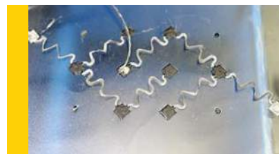
Demonstrator of the stretchable and wearable enzymatic biofuel cell (BFC).
