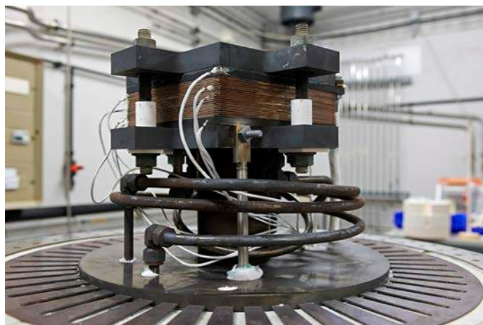
← Solid Oxide Cell stack
